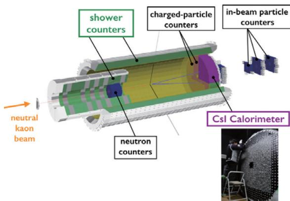
Fig. 1. Schematic drawing of the detector for the KOTO experiment.
